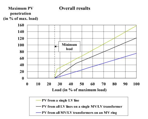
Figure 14 Overall limits of PV penetration into existing power systems
