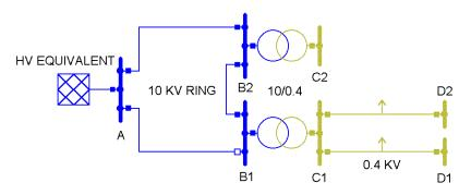
Figure 8 Typical configuration of the MV/LV power system
